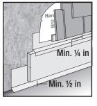
Figure 11 Mortar/Masonry
