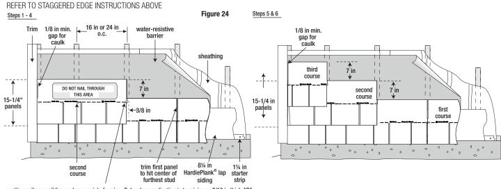
position nails on nail line and secure into framing. Only when application is to minimum 7/16 in thick APA rated sheathing, position nails on nail line spaced a maximum of 13 3/4 in o.c. Allow 3/8 in from panel edges.
