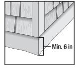
Figure 9 Gutter to Siding
