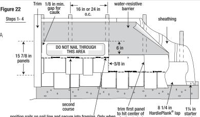
position nails on nail line and secure into framing. Only when furthest stud siding state application is to minimum 7/16 in thick APA rated sheathing, position nails on nail line spaced a maximum of 13 3/4 in o.c. Allow 3/8 in from panel edges.
