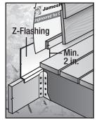
Figure 8 Ground to Siding
