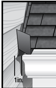
Figure 9 Gutter to Siding
